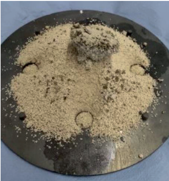
Fig.3: Formed Agglomerates and bed material after a test run [27]
