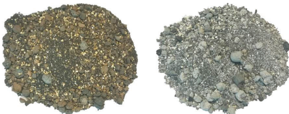
Fig.8: Bed material ash mixture from the combustion reactor entering the gasification reactor (left: brown-red colored) and leaving the gasification reactor (right: gray colored)
