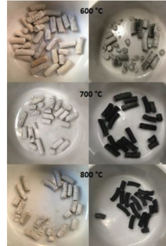
Fig. 8: Samples 1-6; Combustion with (left) and without (right) preheating step
